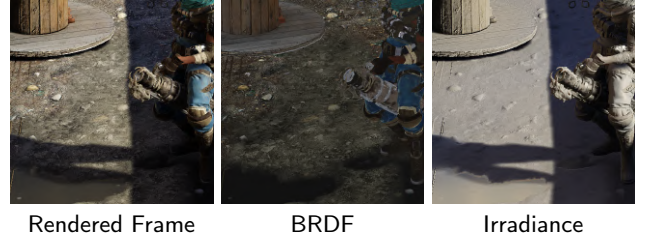
Figure 3: Illustration of BRDF demodulation. The shaded frame is factorized into BRDF and irradiance. This separation shifts the network’s learning focus to low-frequency lighting while high-frequency reflectance patterns are reapplied during remodulation.
